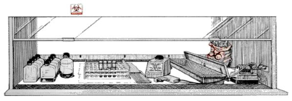
Figure 1. Arrangement of materials in a BSC, with "clean" items separated from "dirty" materials. Source: *BMBL*, 5<sup>th</sup> Edition
