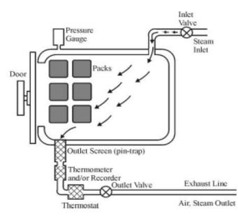
Figure 3. Autoclave diagram.
